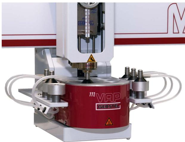
**Figure 2.** GERSTEL Multi-Position Evaporation Station (<sup>m</sup>VAP).
