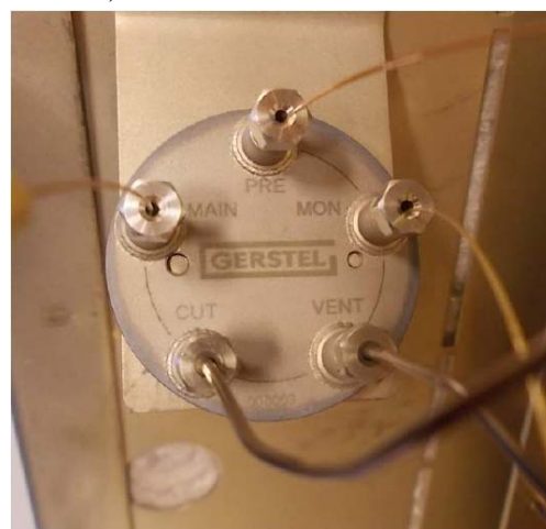
Figure 2. GERSTEL µMCS fraction distribution device.
