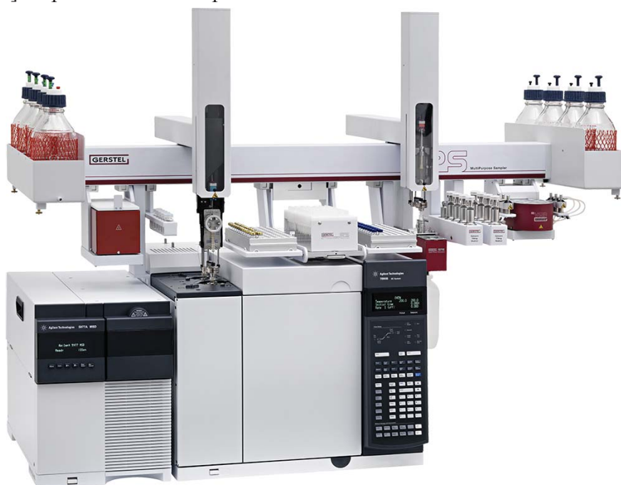
Figure 1. Setup used for the automated analysis of blood serum for THC and metabolites. Dual Head MultiPurpose Sampler (MPS) equipped with solvent bottle holder, agitator, standard wash station, trays for eluate vials, SPE cartridges and samples, SPE module, two solvent filling stations (SFS), MultiPosition eVAPoration station (mVAP) and solvent bottle holder (from left to right).
