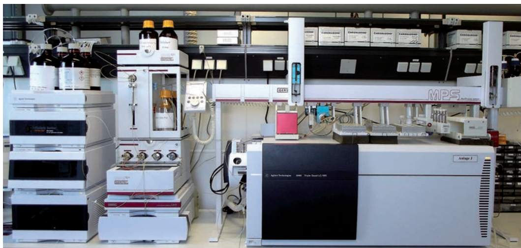
The SPE XOS -HPLC-QqQ-MS system used for the determination of phenylurea and triazine herbicides.
