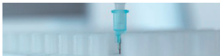
Figure 3: Picture of the MPS picking up a 0.45 µm filter from the filtration tray.
