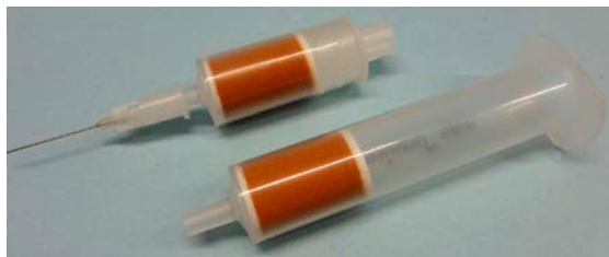
Standard solid phase extraction cartridge (bottom) adapted for automated SPE.
