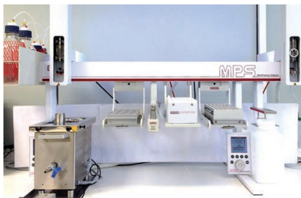
Figure 1: MPS Dual Head WorkStation configured for automated ultrasonic extraction and filtration.
