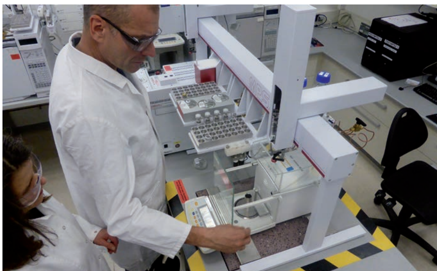
When they prepared their laboratory restructuring, Schülke & Mayr focused on automated sample preparation. Mr. Teevs and his team specifically wanted an autosampler with integrated weighing option that can dispense a wide range of volumes accurately and efficiently without time-consuming syringe changes while offering the possibility to monitor, control and document the dispensed volumes. They found all this and more in the GERSTEL MultiPurpose Sampler (MPS).
